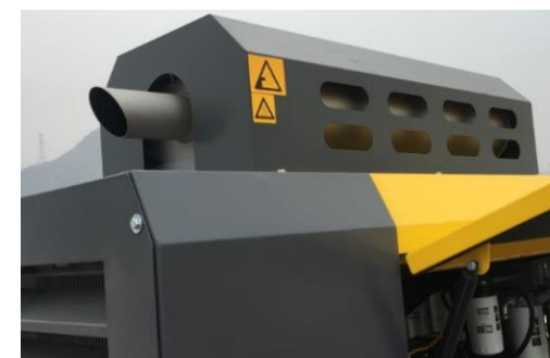
Top mounted muffler for less fire risk and heat load
