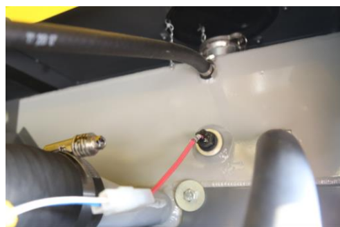
Integrated top tank with radiator: less risk for leakage and corrosion
