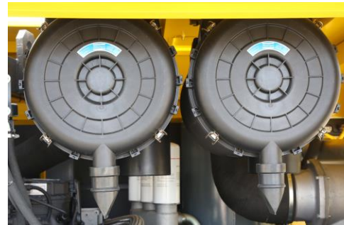
Heavy duty air filter with safety cartridge as standard
