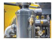
Water separator with level switch (one individual separator per stage) and metal braided airline hoses as standard.
